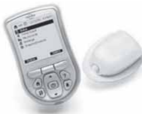
Fig. 1. The OmniPod® insulin patch pump comprises a personal data manager (PDM, left) and a tubeless pump/reservoir unit (Pod; right).
